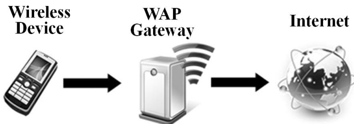
Fig. 1.16. WAP connection through WAP gateway.
